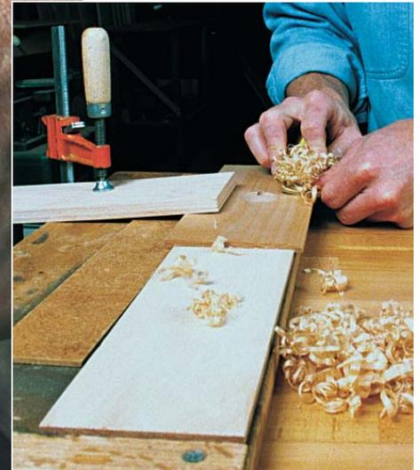
**Shaping the top.** The author uses a bench hook and a block plane (above) to round the top to a fair curve.
