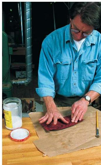
**Polyurethane finish acts as glue.** The author brushes a coat of polyurethane onto a sheet of rice paper and the box bottom, then lays the paper on the bottom and lets it dry.
